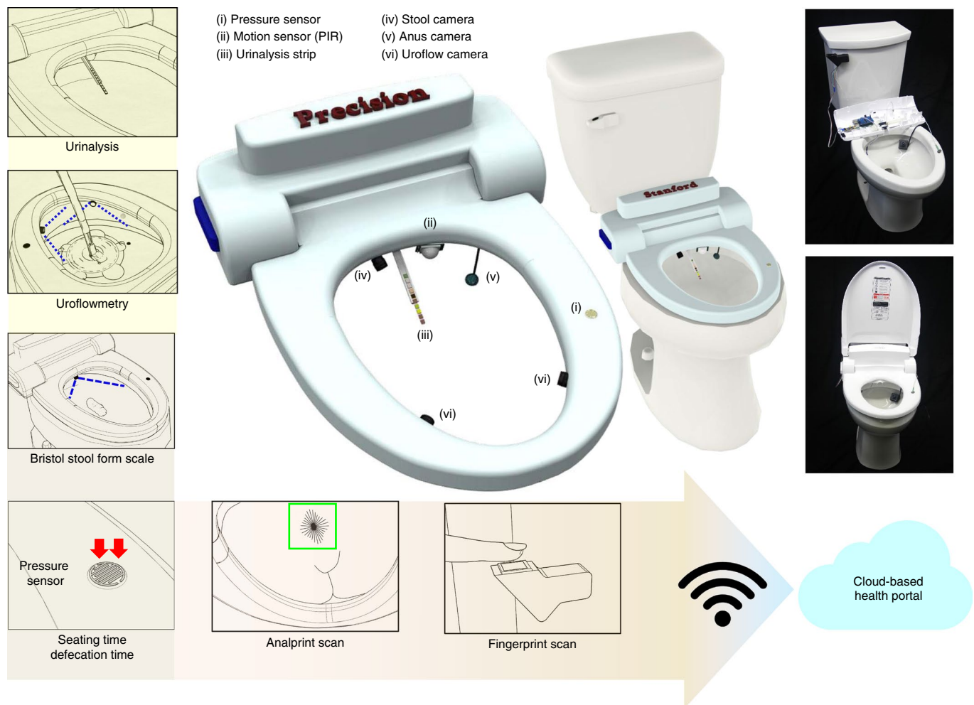
Fig. 1 | Schematic of the toilet system. A perspective view of a toilet with a mountable device for continuously measuring baselines of human excreta. The toilet system includes (1) a 10-parameter test-strip-based urinalysis with a retractable cartridge; (2) computer-vision uroflowmetry with two high-speed cameras (the blue dotted lines represent the FOV from each camera); (3) stool classification by deep learning (the blue dotted lines represent the FOV of the defecation monitoring camera); (4) defecation time measurement detected by a pressure sensor below the toilet seat (the red arrow represents the force applied to the pressure sensor); (5) two-biometric identifications, an analprint scan (the green box represents the template-matching algorithm) and a fingerprint scanner on the flush lever; and (6) the ability to transfer all data by wireless communication to a cloud-based health portal system. Right: photographs of the actual system mounted on a toilet.
